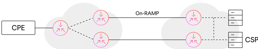
Option 2: A single physical port and dual cloud connections provide full redundancy from Arelion's backbone onward
