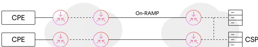
Option 3: Dual physical ports and dual cloud connections provide full redundancy from customer's network onward
